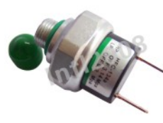
INTL-Y003 M11-P1.0 Male HP:31.4kg/cm 2 Off LP:2.0KG/Cm 2 Off R-12 R-134A
