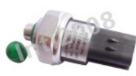
INTL-Y010 Hyundai 3/8-24 UNF Male HP:3.14Mpa Off MP:1.77Mpa On LP:0.196 Mpa Off HFC-R134A 4Pin
